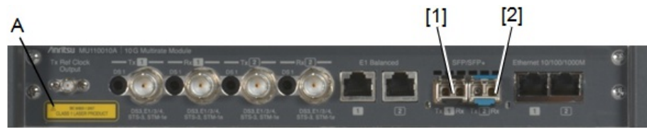
Figure 1: Locations of laser beam aperture (MU110010A)
